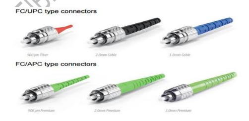
FC fiber optic connectors are designed with cylindrical metal coupling nut with keyed sleeves. Singlemode and multimode FC are with ferrule length at 10.5 ±0.05mm. various color boots are provided in 0.9, 2.0, 3.0mm
