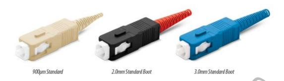
SC fiber optic connectors are with one piece construction and pull-proof design for easy insertion and consistent connection. It has precision anti-rotation key and corrosion resistant body. SC connectors is the most common connector type on the patch panels. SC fiber optic connectors are available duplex and simplex with APC, UPC with ferrule length at 10.5 ±0.05mm.
