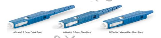
The MU fiber optic connector is about half size of SC with square shape and push pulling mating mechanism. The connector features a pre-assembled body and precision molded plastic housing, and a free floating ferrule measuring 1.25mm O.D. held in place with a precision spring.
