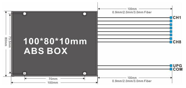
**Note:** Fiber diameter can be 0.9mm/2.0mm/3.0mm. Fiber length is 1M or others. Connector can be LC/SC/FC, or others. If you want to order, please check with us first.
